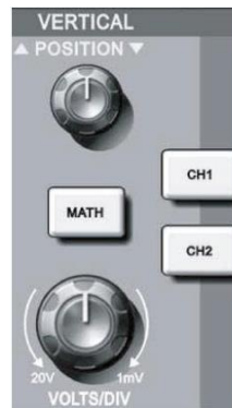
Figure 1-6 Vertical Control Area on the Panel
